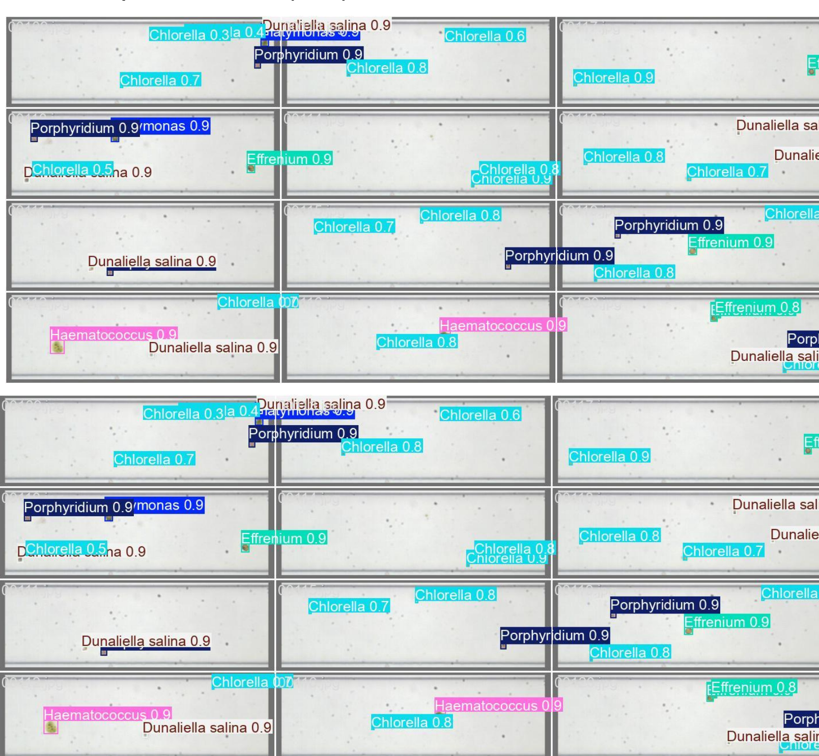
Figure 7 (Left): Outputs from YOLOv8n.pt run for 1000 epochs undertaking object detection and classification (probabilities shown on each cell label).
